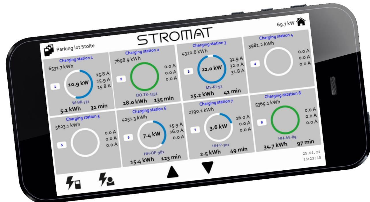
With the **integrated load management**, all connected charging stations are **dynamically controlled** in terms of their electrical output in such a way that the total mains connection is **distributed evenly** to all electric cars.
